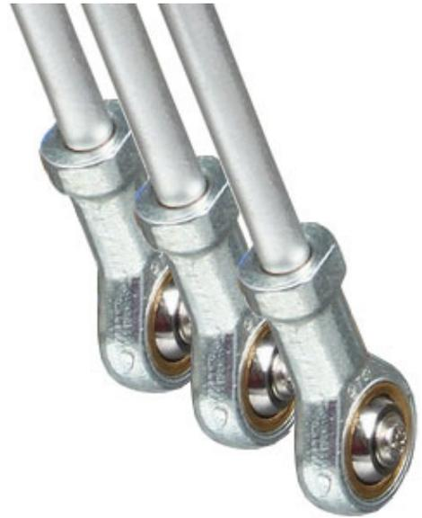
The Diagonal rods are the weak point of the printer kit. All six rods had a different length. I noticed this first after I mounted the delta triangle to the delta towers and the triangle was far from being parallel to the printing bed. From other users I read that this is a common issue. And I just can confirm that. I had differences of up to 2.5 mm in the length of the diagonal rods.
