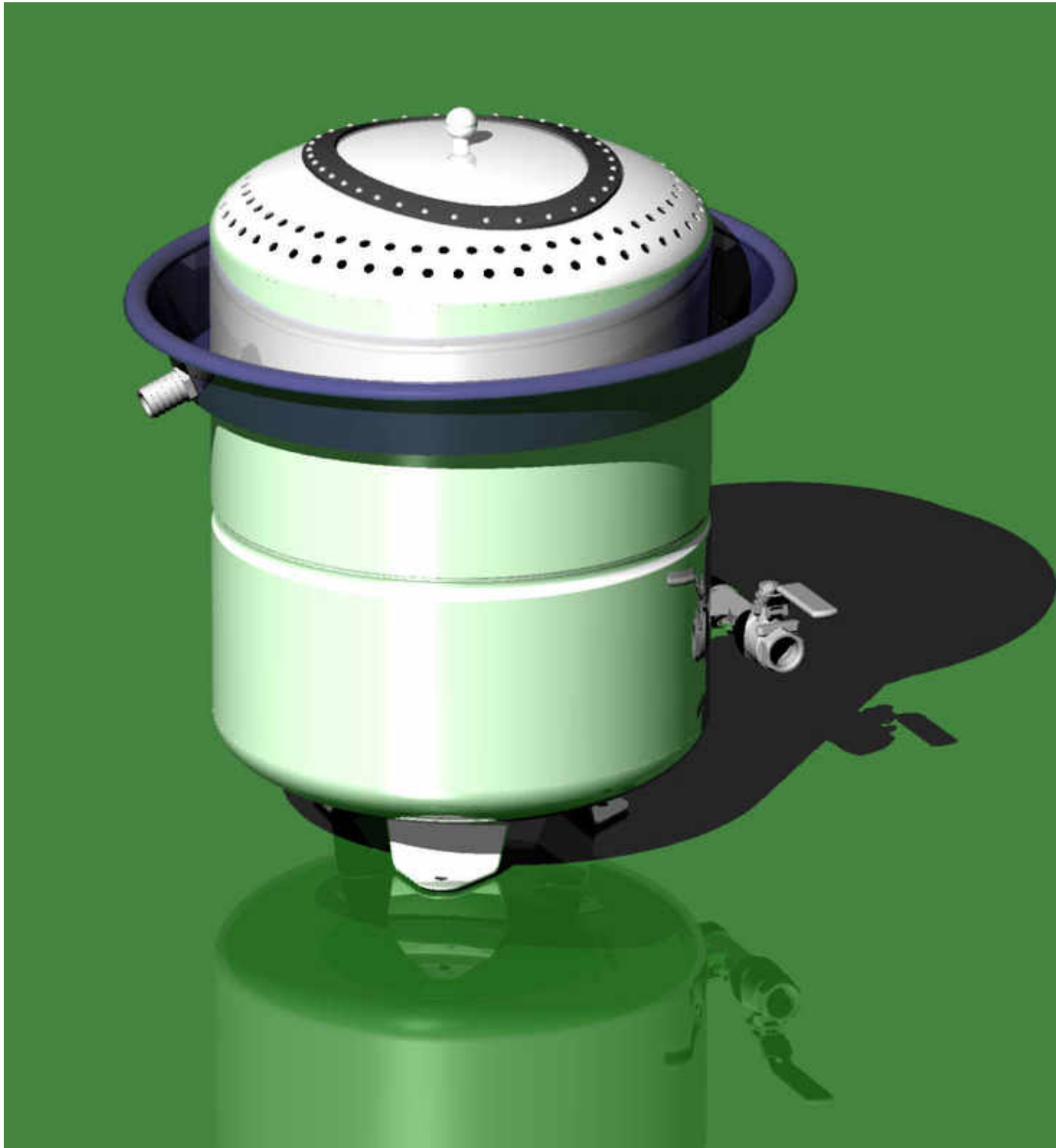
Hydraulic wine press made out of a surge tank
